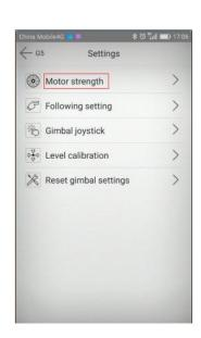
compatible camera. If you added extra lens or there is little vibrations after power on, please kindly increase or decrease the motor strength in 5 by 5 to right setting.
